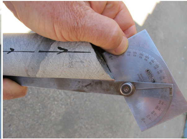
Metal pivoting-arm protractor used to measure alpha angles of bedding (left) and cleavage (right). This type of protractor is by far the most precise (direct measurement to 1 degree) and I have found it very easy to use.
