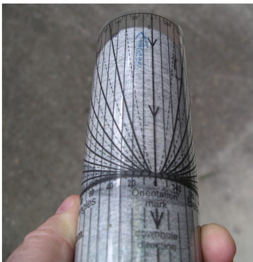
Base of the protractor alpha angle curves aligned with the base of a bedding ellipse.
