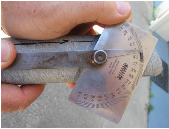
Metal pivoting-arm protractor used to measure alpha angles of bedding (left) and cleavage (right). This type of protractor is by far the most precise (direct measurement to 1 degree) and I have found it very easy to use.
