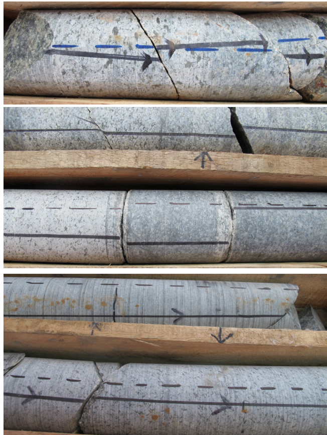
Examples of incorrectly drawn BOH line (black) by a driller's offsider in a single short interval of core.
